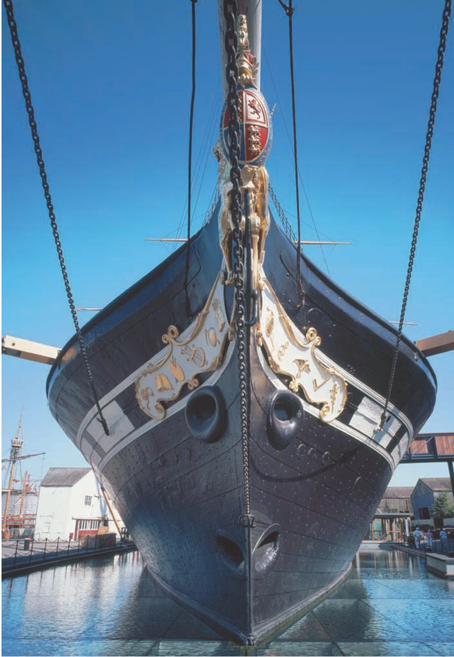
7, 8 The SS Great Britain – now converted into a visitor centre – in the dry dock at Bristol, where the ship was built between 1837 and 1842. The roughly 1000 m 2 waterline plate on which the boat seems to float seals the hull to the edge of the dry dock. Large areas of the visitor centre are housed beneath the 5 cm deep layer of water and the supporting glass roof.
